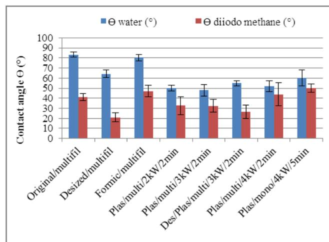
Figure 1: Graphical representation of contact angle measurement
