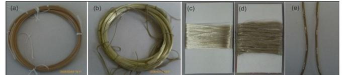
Figure 3: a) Original monofilament, b) silver coated monofilament, c) original multifilament, d) silver coated multifilament and e) unevenness in monofilament in spool wound silvering method.
