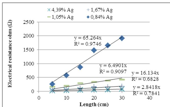
Figure Error! No text of specified style in document.: Graphical representation on the resistance of silver coated PEEK monofilament in respect to length
