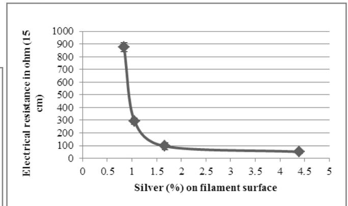
Figure 4: Influence silver content on electrical resistance of monofilament PEEK
