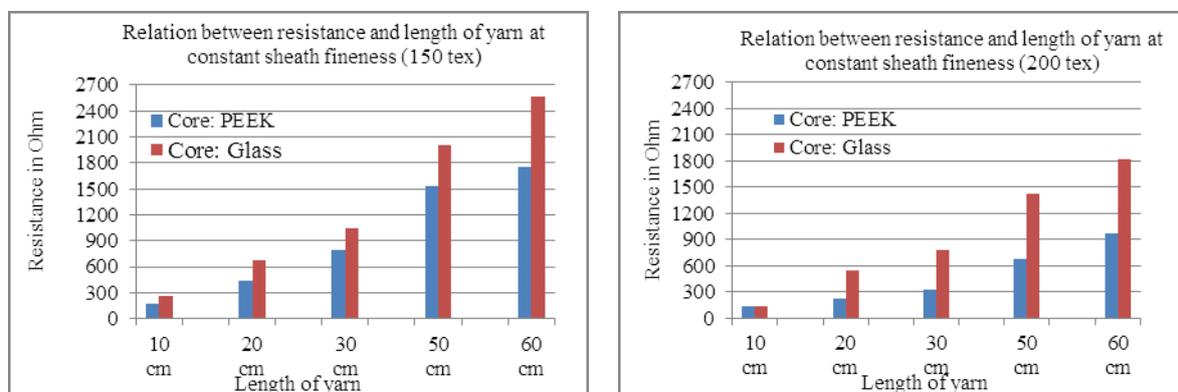
Fig. 6 Relation among resistance, length, sheath and core of hybrid yarn
