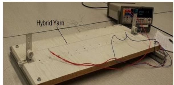
Fig. 4 Method of measuring electrical resistance
