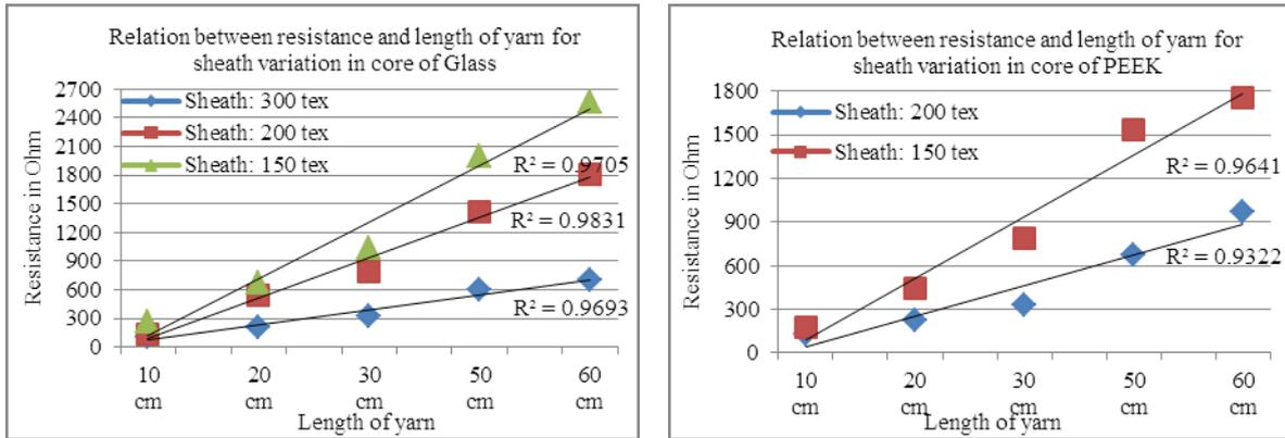
Fig. 7 Relation between resistance and length of hybrid yarn at different sheath fineness for two different core filament yarns.
