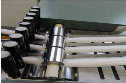
Fig. 3 Feed of slivers in draw frame for first passage
