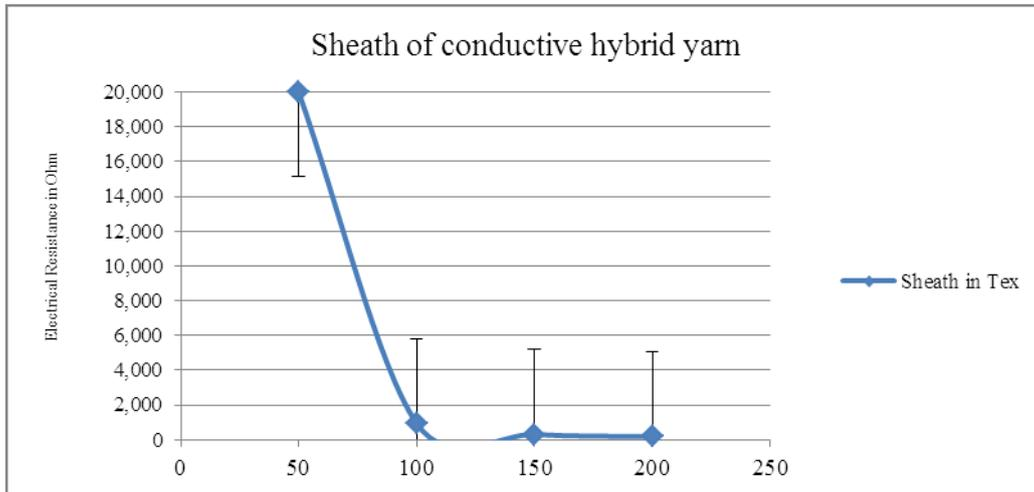
Fig. 8 Relation between electrical resistance and amount of steel fibers in sheath when core is PEEK and sheath is steel with polyester.
