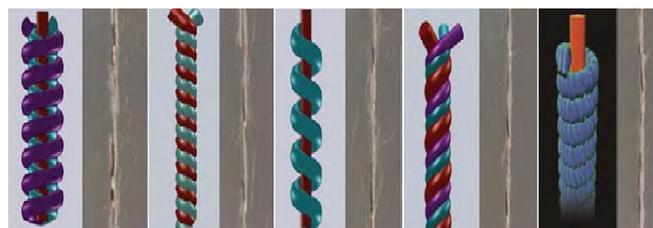
Fig. 2 Structure of hybrid yarn
