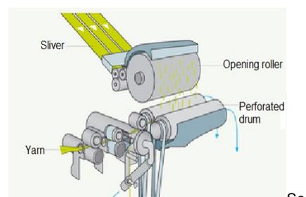
hematic diagram of friction spinning
