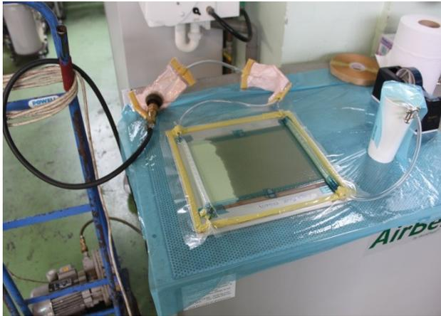
Fig. 2 Resin infusion using vacuum bagging
