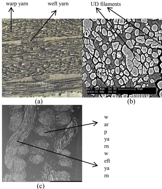
Fig. 6 Microscopic image of different composites; (a) glass fibre composite; (b) UD tape flax; (c) matt fabric flax
