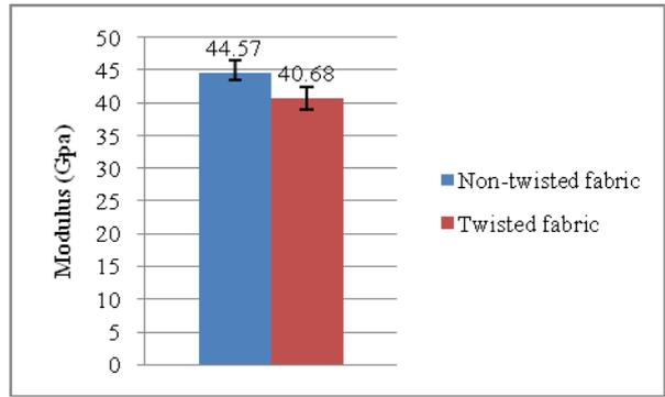
Fig. 3 Modulus of Glass-reinforced composites
