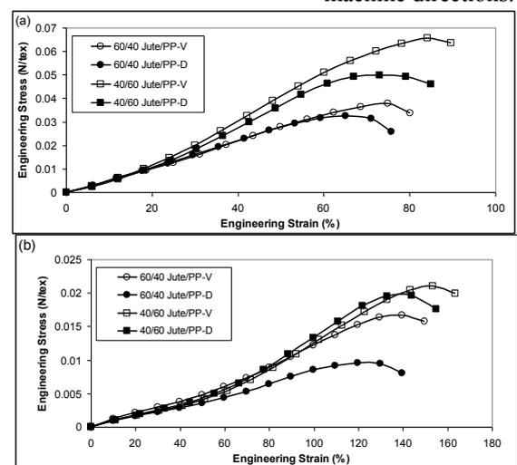
**Figure 2:** Typical stress-strain curves of virgin (V) and damaged (D) needlepunched nonwoven geotextiles (40/60 Jute/PP and 60/40 PP/Jute) (a) cross-machine direction (CD) and (b) machine direction (MD)
