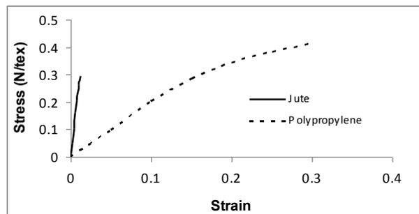
**Figure 1:** Typical stress-strain curves of jute and polypropylene fibres
