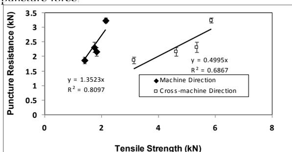
**Figure 3:** Relationship between puncture resistance and tensile strength in cross-machine directions (here error bar indicates standard deviation for puncture resistance)
